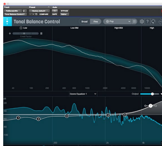
iZotope Tonal Balance 2 In Fine Mode Showing Direct Controls in Ozone 9's Equalizer
